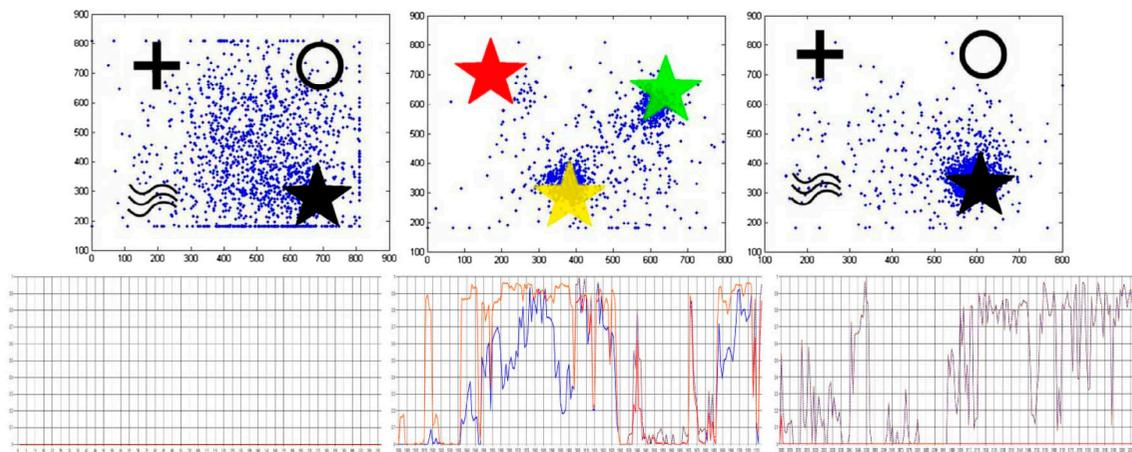
**Figure 5.** From left to right the results of the three phases of the first experiment; blue dots represents where the robot was pointing at, red and blue signals are, respectively, from the IM and the GM.
