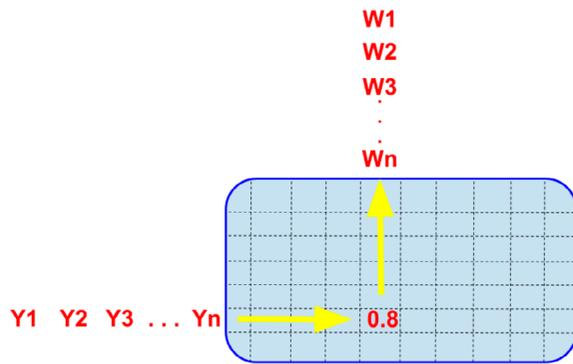
**Figure 4.** The State-Action Table;  $Y_1, \dots, Y_n$  represents the actual state,  $W_{m1}, \dots, W_{mn}$  are the weights for movement generation; each entry is the reward of the action, i.e. the Relevant Signal.
