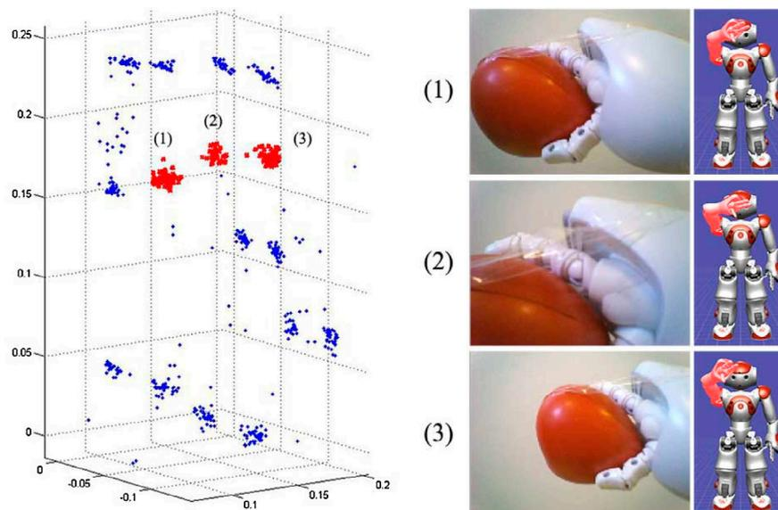
**Figure 6.** In the three-dimensional (3D) graph blue dots represent the positions of the right hand at each cycle, while in red are highlight those corresponding to good positions (as shown in the right part of the image); the higher concentration of dots in these three areas demonstrates that the robot has learnt various movements to accomplish its goal.
