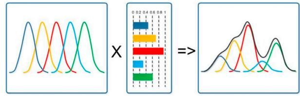
**Figure 3.** Motor primitives composition: each Gaussian function is a motor primitive; the weighted sum of all these primitives is the final movement; learning a movements is thus learning an optima set of weights.
