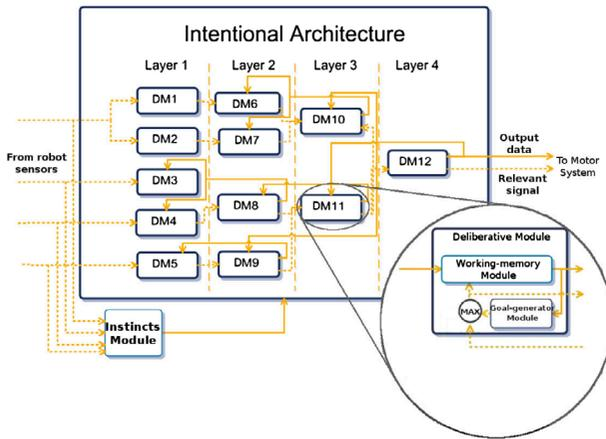
**Figure 2.** Several DMs are interconnected in a layered network; each DM is composed by two sub-modules: WM and GM; a IM feed each DM with an emotional signal.
