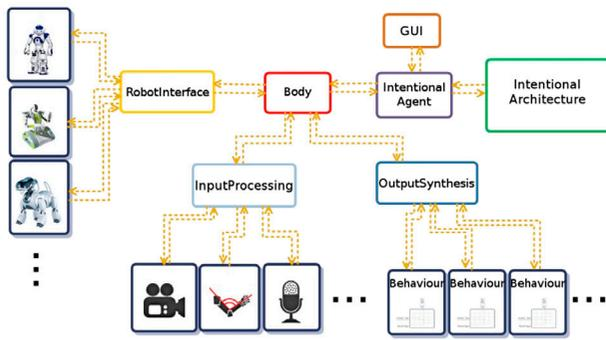
**Figure A1.** An abstraction of the UML diagram of the IDRA architecture.
