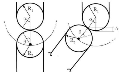
Fig. 4. The upward movement can be expressed as a function of  $R_1$ ,  $R_2$  and the rotation  $\theta$ , due to the constrain of rolling without slipping.
