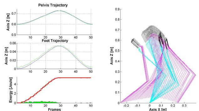
Fig. 9. Energy consumption with minimum height for pelvis at 0.55m
