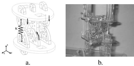
Fig. 2. (a) The knee joint designed for our robot. The arrows show the way the tendons are wrapped. (b) The knee prototype
