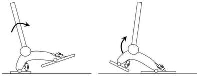
Fig. 7. The foot developed to mimic the human one. It has two passive degrees of freedom, and a spring-damper system to smooth the heel-strike
