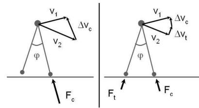
Fig. 5. In the figure,  $v_1$  and  $v_2$  are the  $cm$  velocities respectively before and after heel-strike, while  $F_c$  and  $F_t$  are the ground reaction forces. With toe off (on the right) the  $cm$  vertical velocity is reduced, and the gait is smoother and more efficient.
