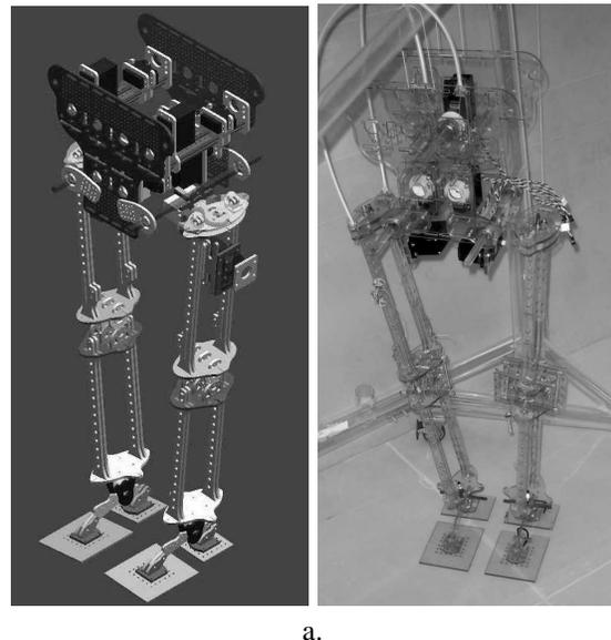
Fig. 1. (a) The 3D cad assembly of the robot. (b) The prototype, here with only one leg actuated.
