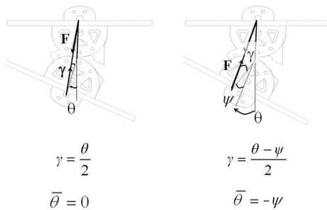
Fig. 3. We can exploit the action of the springs to impose a suited torque on the joint. In particular, it is possible to generate a position of instable equilibrium ( $\theta = \bar{\theta}$ ) to favor knee bending and stretching.
