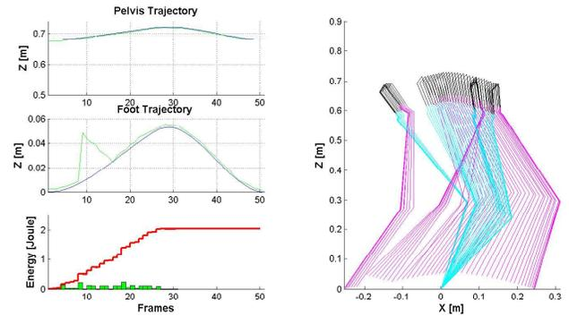
Fig. 8. Energy consumption with minimum height for pelvis at 0.68m
