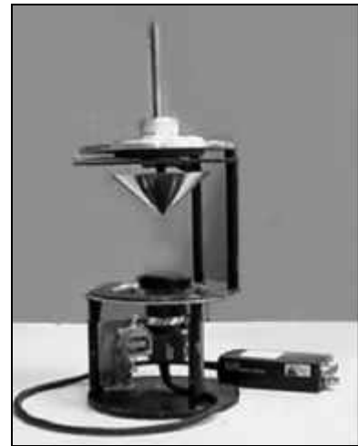
Figure 7. The omnidirectional sensor with the conical mirror.
